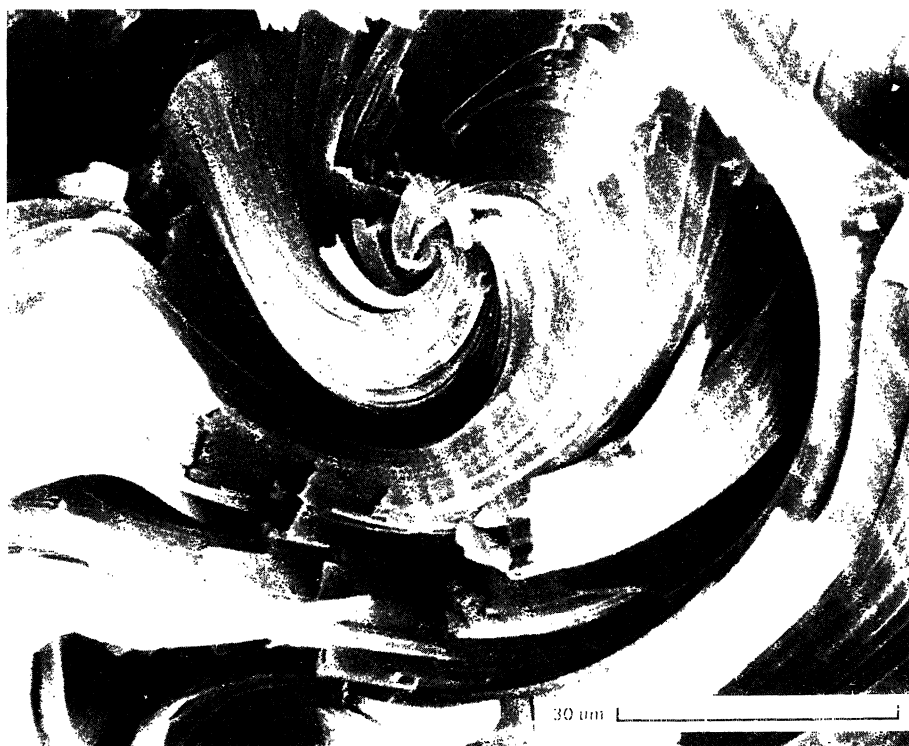
Figure 19. A fracture surface of a liquid crystalline polymer (random copolyester of 75% hydroxybenzoic acid and 25% hydroxynaphthoic acid) of molecular mass 5000. The director trajectory, as revealed by the directional fissility, would suggest the intersection of an s = +1 disclination with the surface.
